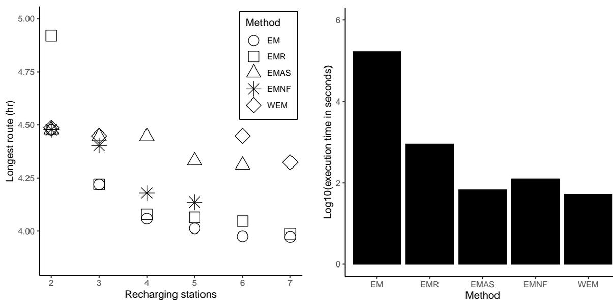
(a) Pareto optimal front and the fronts returned by the proposed approaches. (b) Logarithmic scale of the time to compute the fronts.
