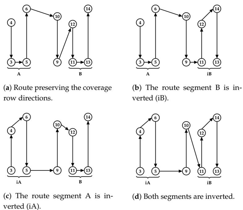
Figure 8. Example of routes generated by changing the coverage row directions.
