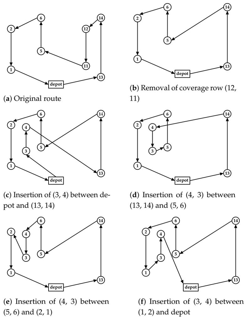
Figure 7. Example of link evaluation heuristic performed on Swap to compute the route.
