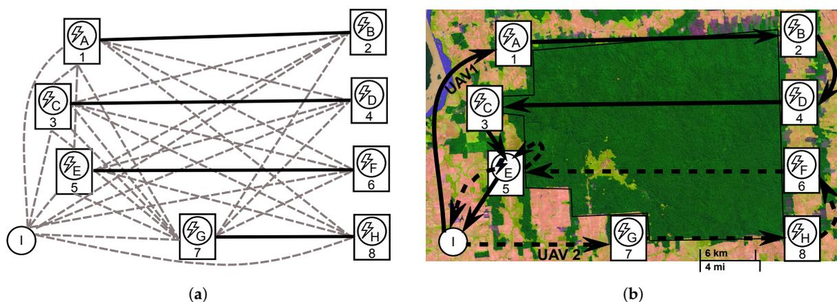
**Figure 1.** Example of the graph used to represent a coverage area and the solution illustrated in a preservation area image. (a) The recharging stations that can be opened in the area are represented by A–H, the depot is the vertex (I), and the targets are identified by the numbers 1–8. (b) An illustration of coverage routes applied to preservation area monitoring. Deforestation map of the Amazon from the TerraBrasilis website [68].
