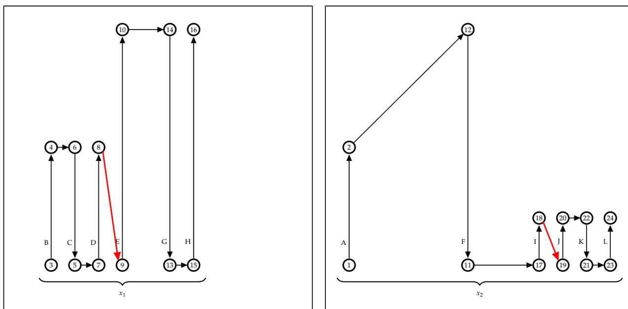
(a) Initial route for  $x_1$  linking the subroutes  $x_1^1 = \langle 3, 4, 6, 5, 7, 8 \rangle$  and  $x_1^2 = \langle 9, 10, 14, 13, 15, 16 \rangle$ .
