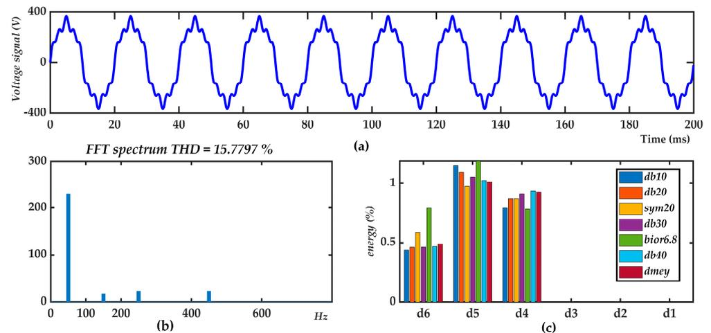
**Figure 2.** Voltage signal with harmonics: (a) Instantaneous representation, (b) FFT spectrum, (c) distribution of the energy percentage of the signal according to the coefficients of the mother wavelets.
