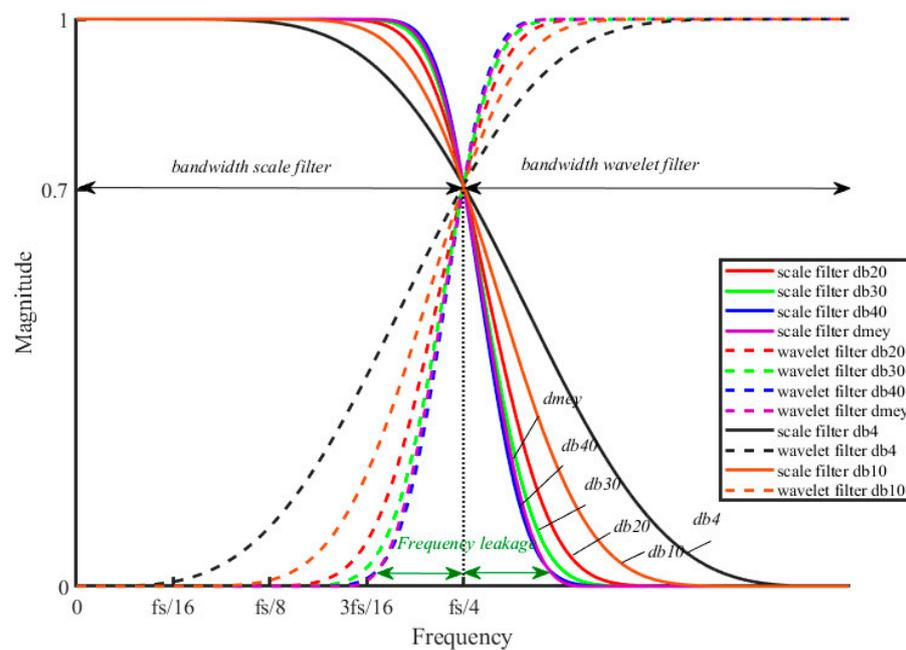
**Figure 1.** Comparative frequency response of mother wavelets.
