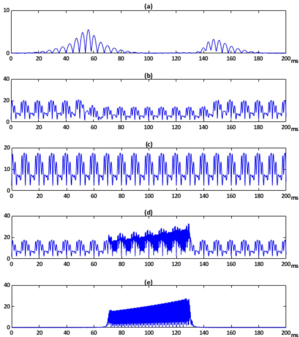
Figure 9. Instantaneous Transient Disturbance ratio index  $ITD(t)$  of voltage disturbances combination.
