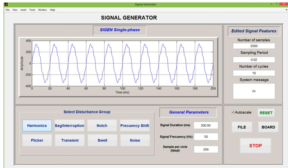
Figure 4. Graphical user interface of the *Sigen* system.
