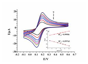
Fig. S2 Cyclic voltammograms of the bare electrode at different scan rates (0.025 V/s, 0.050 V/s, 0.075 V/s, 0.100 V/s, 0.125 V/s, 0.150 V/s, and 0.200 V/s). The inset shows that the redox peak current had a good linear relationship with the square root of the scan rate, indicating that the redox peak current was only controlled by diffusion.
