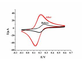
Fig. S1 Cyclic voltammetry characterization before and after the pre-treatment of bare electrode. As shown in Figure S1, the redox peak current increased considerably, the peak current ratio was close to 1, and the peak potential difference was less than 80 mV.
