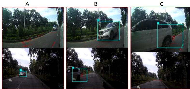
**Figure 3.** Example target tracking and camera switching. (A) Example image set  $I_t$  containing one target in backward camera. (B) Example image set  $I_{t'}$ ,  $t' > t$  containing the same target in the backward and right cameras. The area of the bounding box in right camera is larger than that in the backward camera. At that point, tracking switches from the backward to the right camera. (C) The target has disappeared in the backward camera but is tracked in the right camera.
