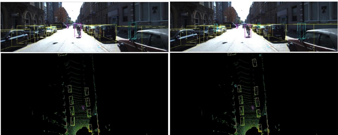
**Figure 9.** Example of a KITTI frame inference results for PTQ (left point cloud top view) and Optimised QAR (right image) configuration 2 model.
