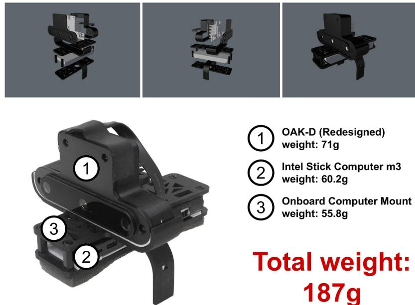
**Figure 5.** The 3D-printed mount to carry the OAK-D smart camera (with the new back case) and the Intel Compute Stick onboard the drone.
