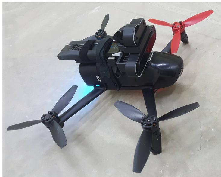
**Figure 3.** First mount design enabling the Bebop 2.0 Power Edition to carry the Intel Compute Stick and the OAK-D smart camera with its original case. In this design, the total weight was 283 g, 117 g for the OAK-D sensor, plus 166 g for the onboard computer and the mount. This exceeds the maximum payload set by us (200 g) by 83 g, which resulted in unstable flights.
