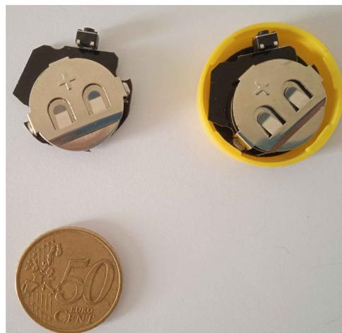
**Figure 5.** Bluetooth tags used during our experiments.
