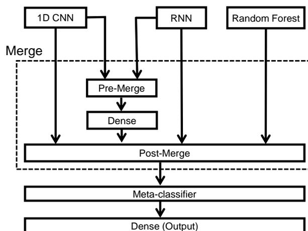
Figure 9. Block diagram of the stacking ensemble learning.
