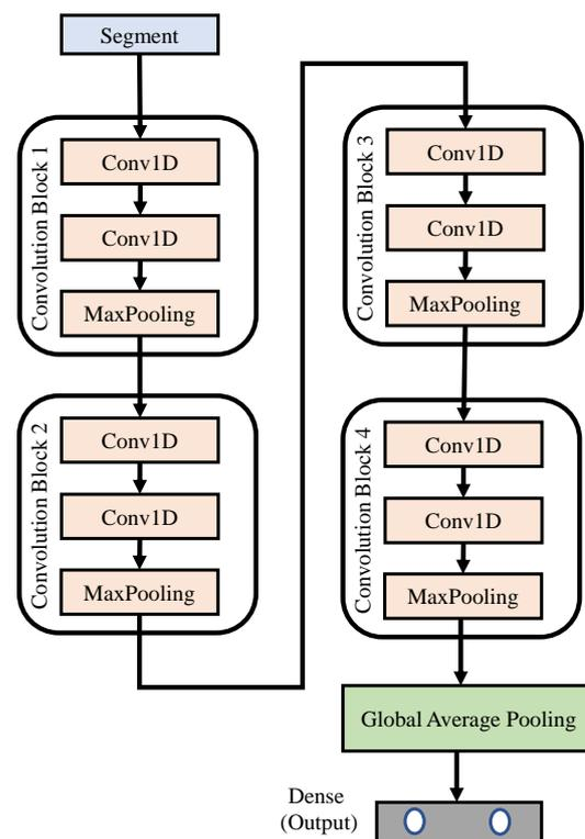
Figure 7. Block diagram of the proposed 1D CNN networks.
