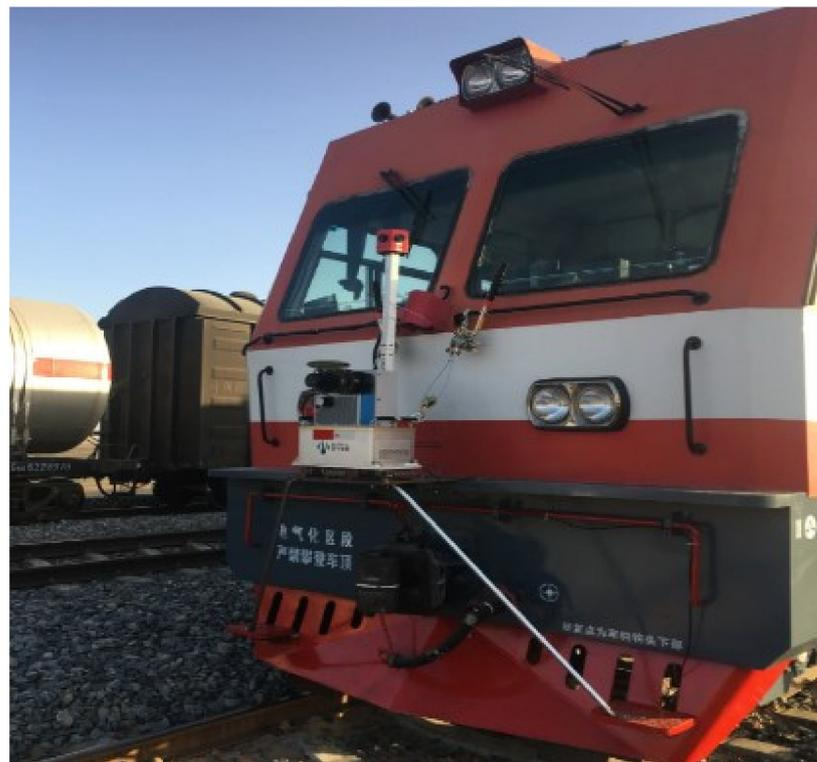
**Figure 4.** Vehicle-mounted LiDAR and its installation location.
