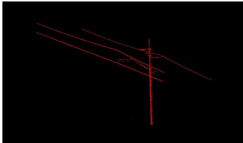
**Figure 6.** Railway OCS point cloud with a length of 50 m.
