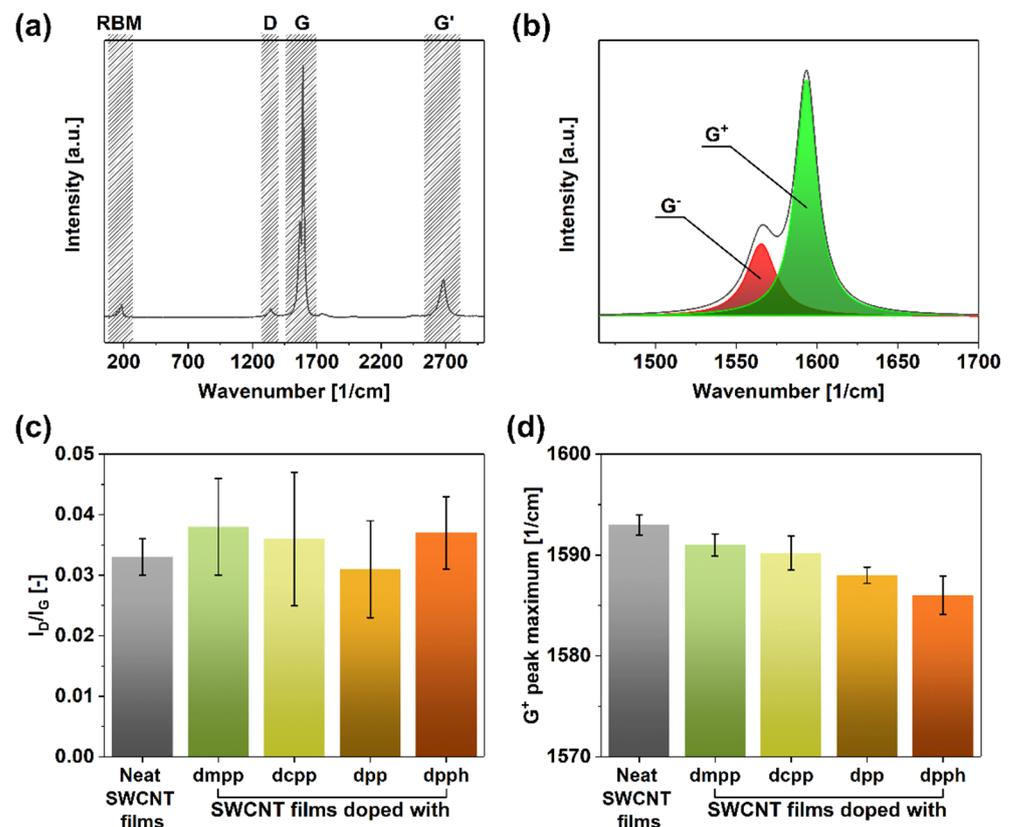
**Figure 2.** (a) Full Raman spectrum of a neat SWCNT film, (b) magnification of the G peak area with exemplary deconvolution into  $G^-$  and  $G^+$  components, (c)  $I_D/I_G$  ratios of SWCNT films before and after doping, and (d) corresponding recorded positions of  $G^+$  peak maxima after deconvolution.
