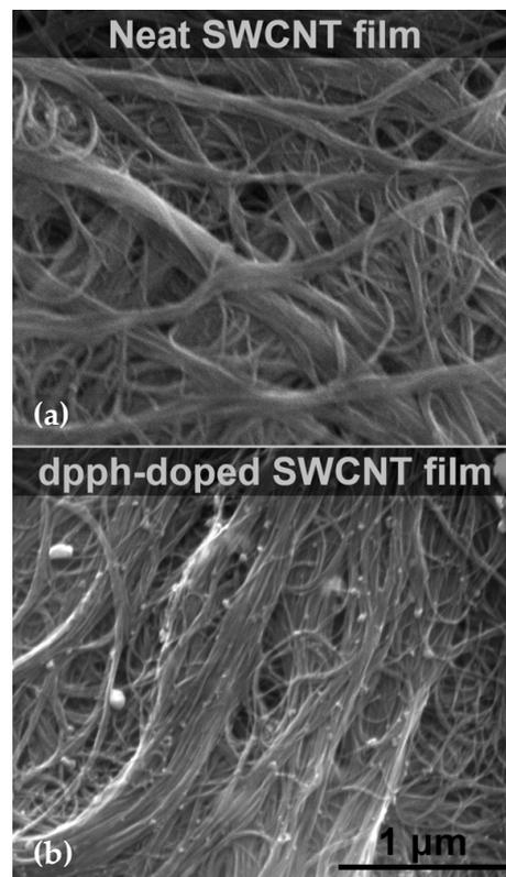
Figure 3. SEM micrographs of (a) neat SWCNT film and (b) upon doping with dpph.
