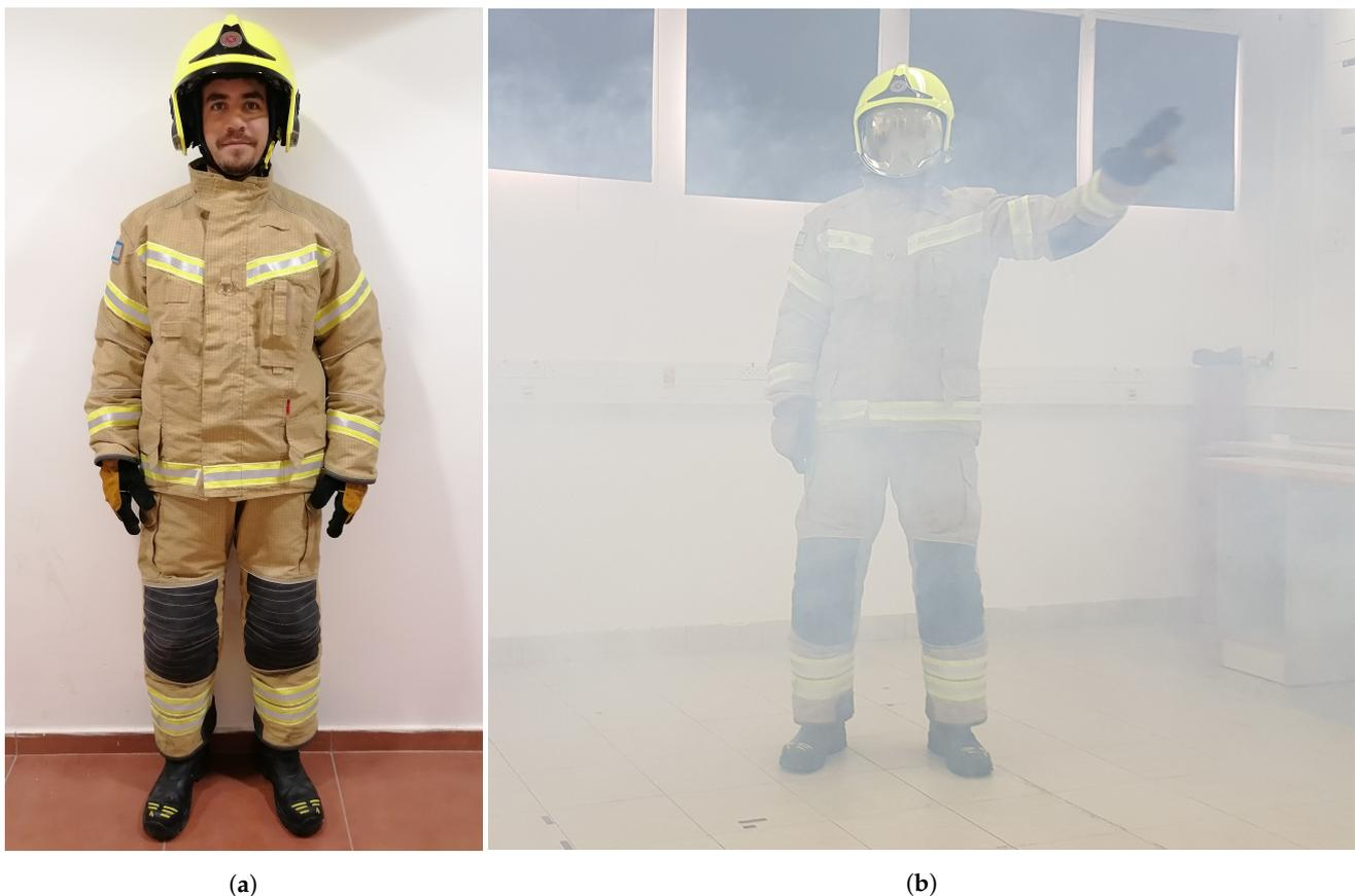
**Figure 6.** (a) Firefighting equipment including helmet, jacket, trousers, and gloves and (b) experiment conducted to evaluate the system's accuracy with full equipment and smoke.
