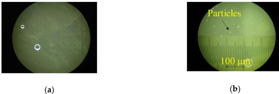
**Figure 3.** Observation results of (a) new and (b) used engine oils using the microscope.
