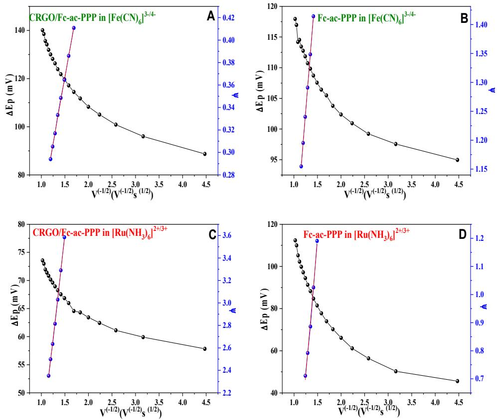
**Figure S5.** Relationship of  $\Delta E_p$  and  $\psi$  versus  $v^{-1/2}$  of Au electrode modified with CRGO/Fc-ac-PPP (A, C) and Fc-ac-PPP (B,D) with  $[\text{Fe}(\text{CN})_6]^{3-/4-}$  and  $[\text{Ru}(\text{NH}_3)_6]^{2+/3+}$  redox marker.
