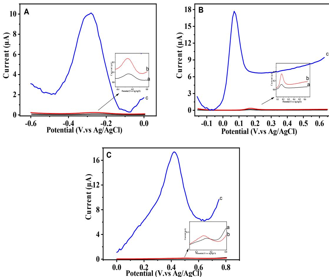
**Figure S6.** DPVs responses of (A) 10<sup>-4</sup> M AA , (B) 10<sup>-5</sup> M DA and (C) 10<sup>-4</sup> M UA at (a) bare Au, (b) Au/Fc-ac-PPP and (c) Au/RGO/Fc-ac-PPP in 0,1M PBS (pH=7).
