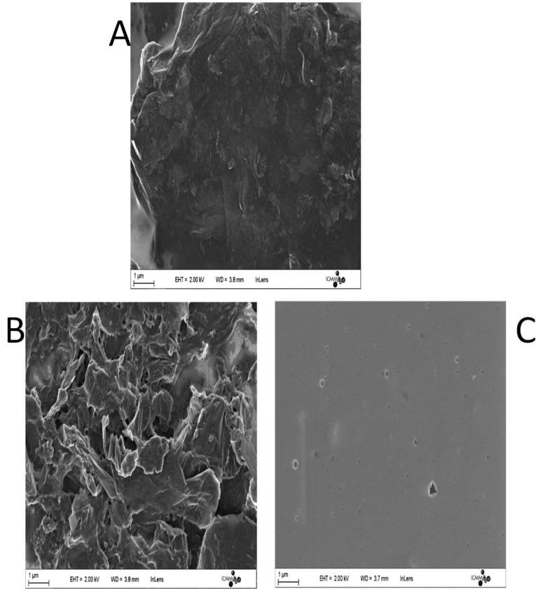
**Figure S3.** Scanning electron microscope (SEM) images of (A) nanocomposite CRGO/Fc-ac-PPP compared to (B) CRGO and (C) Fc-ac-PPP.
