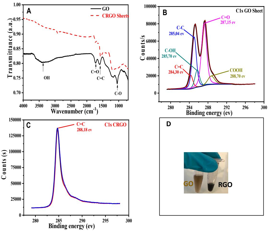
**Figure S1.** FT-IR spectra (A) Fourier transform infrared spectroscopy (FTIR) spectra of GO and CRGO. X-ray photoelectron spectroscopy (XPS) spectra in carbon region of (B) GO and (C) CRGO. (D) Photographs of the GO solution before and after reduction.
