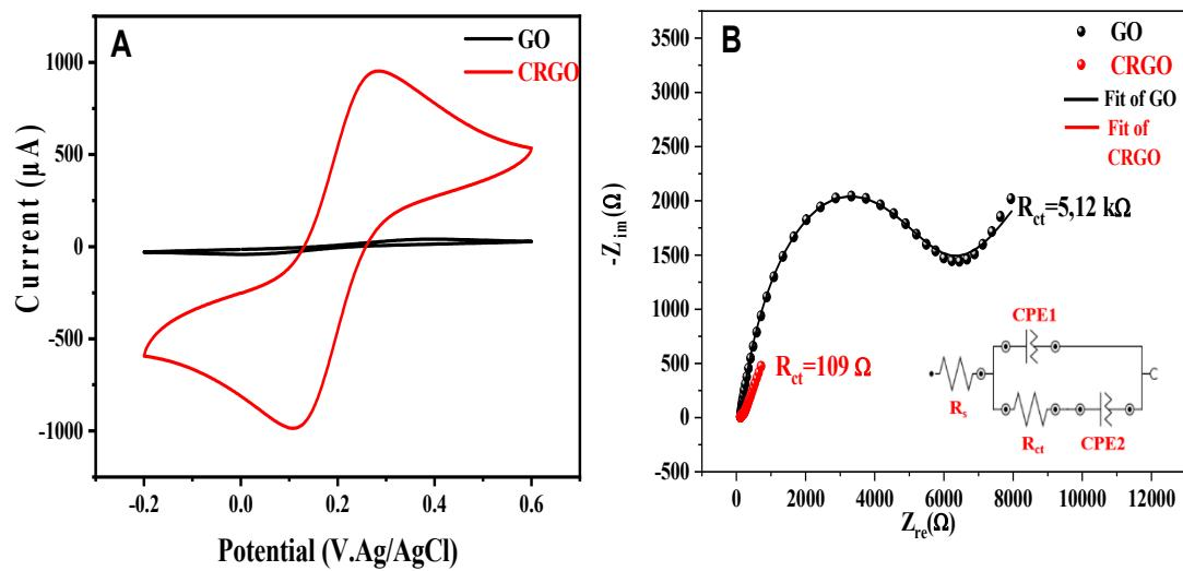
**Figure S2.** (A) Cyclic voltammetry (CV) of GO and CRGO in the solution of 10mM  $[\text{Fe}(\text{CN})_6]^{3-/4-}$  in 0.1M KCL at a scan rate of 50 mVs  $^{-1}$ . (B) Electrochemical impedance spectroscopy (EIS) of Au modified with GO and RGO analyzed in solution of 10mM  $[\text{Fe}(\text{CN})_6]^{3-/4-}$  in 0.1M KCl with amplitude of 10mV and frequency range from 0.1Hz to 100KHz.
