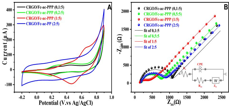
**Figure S4.** (A) CVs and (B) EIS of Au/CRGO/Fc-ac-PPP obtained with different mass ratio analysed in 10mM PBS solution pH=7 free of redox marker. CVs are obtained with scan rate 50mV/s and. EIS amplitude 10mV and frequency range from 100 KHz to 100 mHz.
