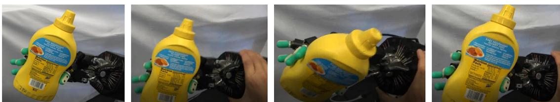
**Figure 13.** Illustration of the object grasping process under the external disturbance exerted by a user.
