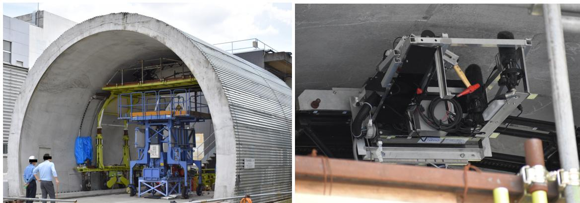
(a) Mock tunnel used in field experiments. Conditions as close as possible of actual inspection sites were realized due to its scale and naturally-occurred defects. (b) Hammering module mounted on Variable Guide Frame. This setup allows automatic collection of hammering samples in any location inside of a tunnel.
