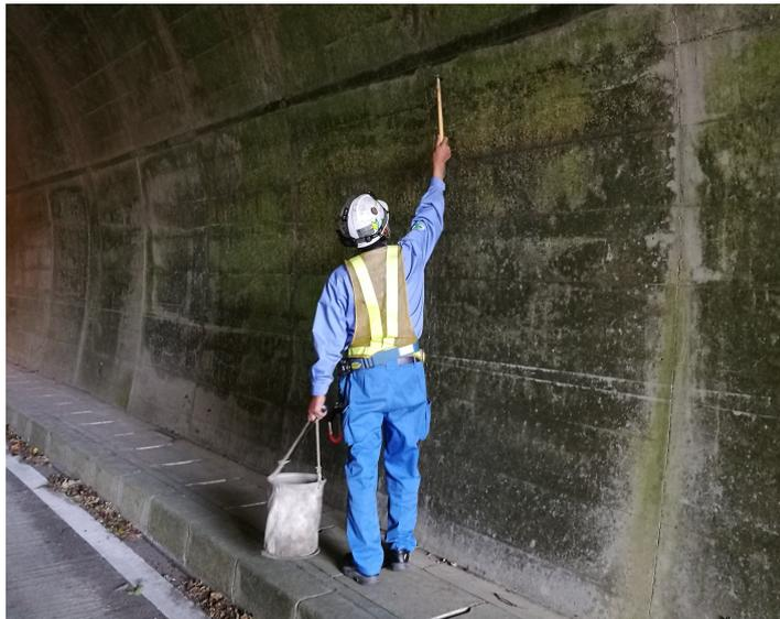
**Figure 1.** Hammering test conducted by a professional on the upper wall portion of a tunnel: only a simple hammer is needed, thus the popularity of this non-destructive testing method. However, there is the need of skilled operators to correctly differentiate hammering sounds and given the great population of structures in need of testing, automation is actively demanded. In addition, since it relies heavily on the operator's skills, the final result remains subjective.
