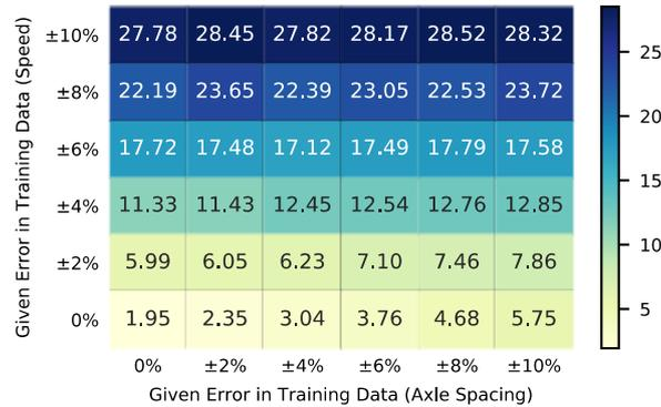
**Figure 11.** Identification error (%) of axle weights of conventional BWIM algorithm with error-included speed and axle spacing information (Two-axle Trucks).
