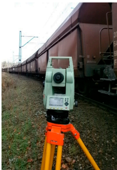
Figure 3. The electronic total station TC-407—measuring station.
