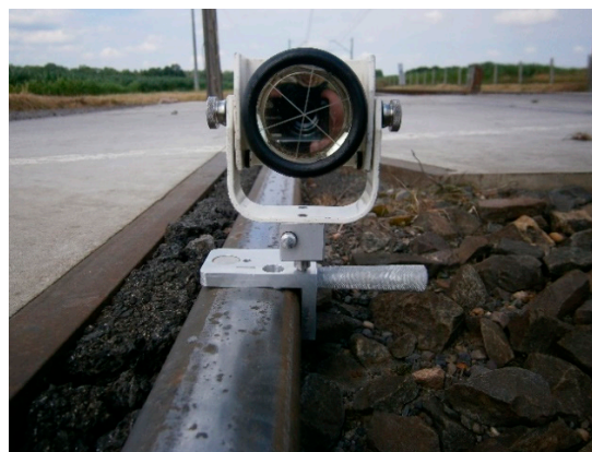
Figure 5. Geodetic standard prism (round) integrated with MMS.
