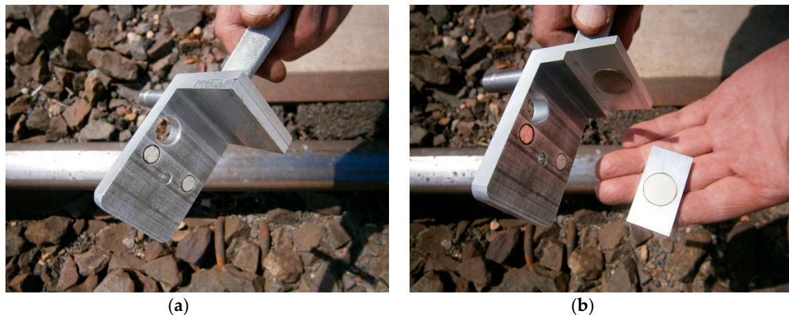
Figure 4. Magnetic base in MMS construction for mounting on metal parts: (a) with a reduction plate; and, (b) without a reduction plate.
