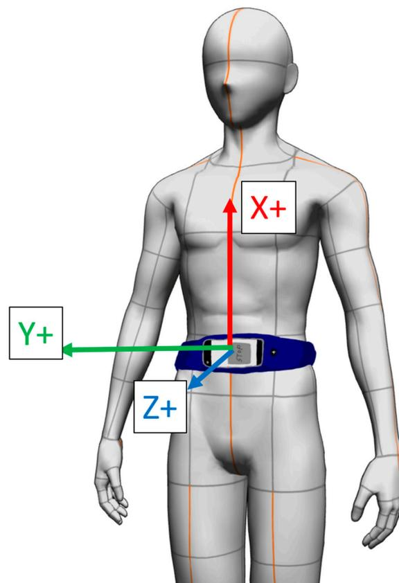
Figure 1. The orientation of the smartphone.
