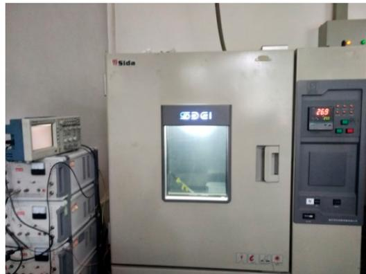
**Figure 3.** The thermostat for RLG temperature experiments.
