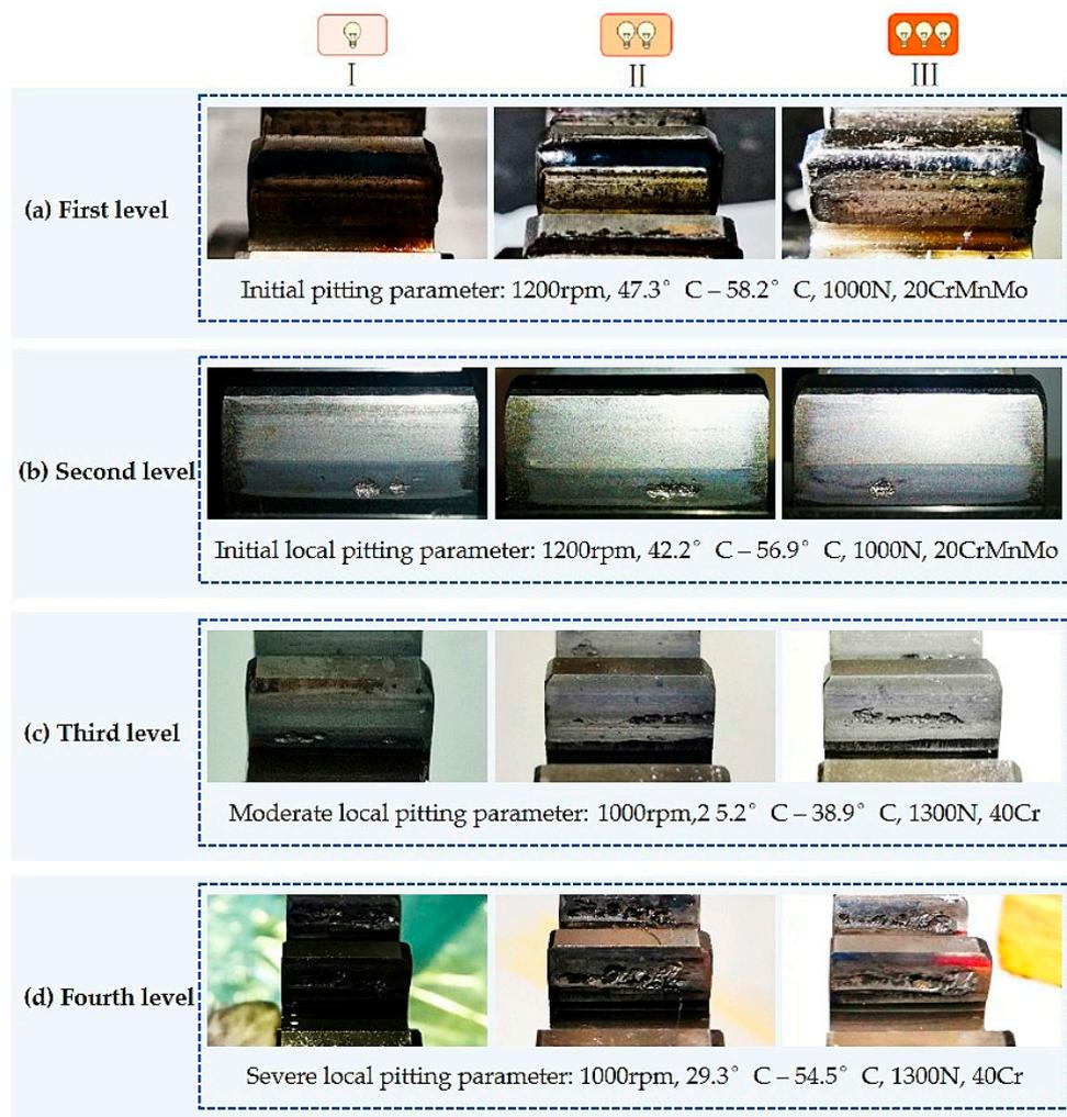
**Figure 3.** Gear pitting images obtained under different levels. According to the area of pitting, pitting was divided into four grades: initial pitting (first level), initial local pitting (second level), moderate local pitting (third level) and severe local pitting (fourth level).
