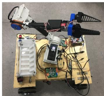
**Figure 8.** Prototype of the picking robot.
