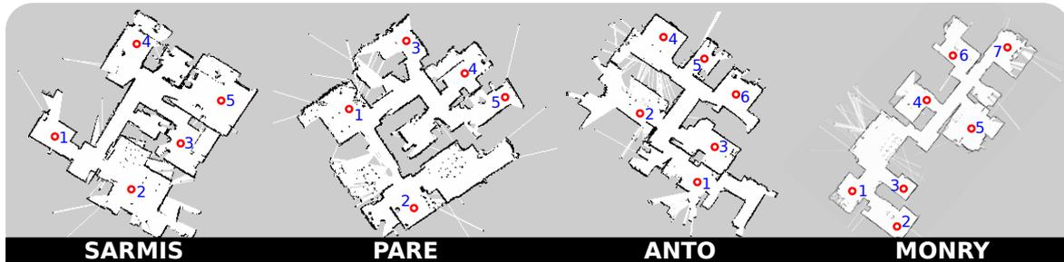
**Figure 4.** Floor-plans of the four houses where navigation will be tested. These geometric maps are built by deploying a mobile robot in the house and teleoperating it while running a SLAM algorithm based on 2D laser range measurements.
