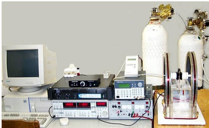
**Figure 3.** The magnetoelastic sensor system. A signal generator sends a pulse-like excitation signal, appropriately amplified, to the interrogation coils. The response of the sensor, located in the white tube placed between the two coils, is monitored with a pickup coil the output of which is passed to a lock-in amplifier. A computer controls the instrumentation and plots measured parameters as a function of time.
