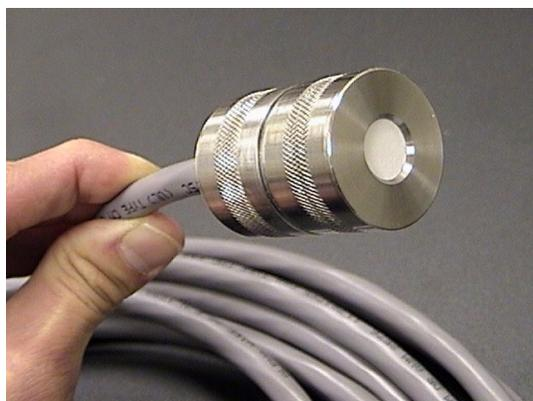
**Figure 3.** Stainless-steel waterproof package that houses the chemiresistor array. A GORE-TEX<sup>®</sup> membrane covers a small window over the chemiresistors.
