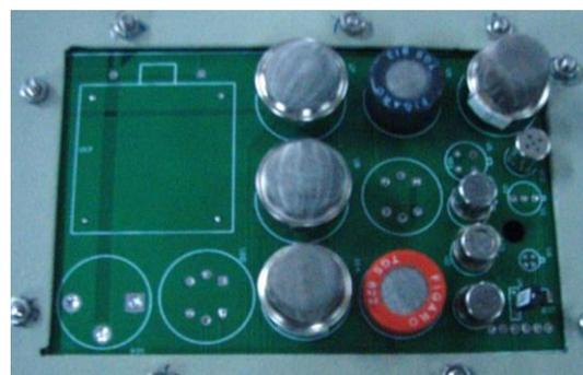
**Figure 3.** The sensors array in the chamber of E-nose.
