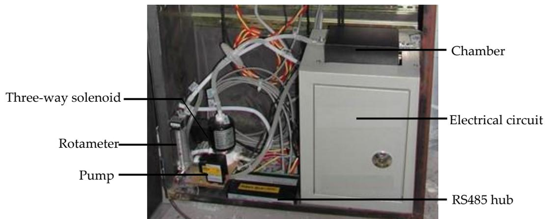
**Figure 2.** Electronic nose (E-nose) prototype.
