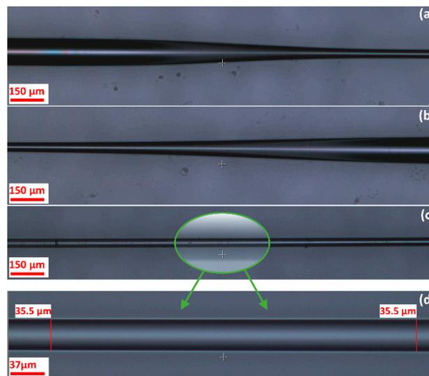
**Figure 4.** (a,b) SMF taper transition, (c) long uniform taper waist, (d) magnified image of the uniform taper waist.
