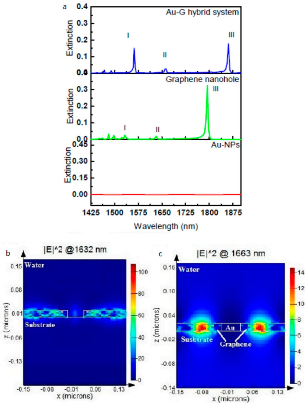
**Figure 4.** (a) Extinction spectrum for three different nanostructures; Au NP square array, nanohole array perforated in 20 nm-thick graphene film, and Au NPs/G hybrid structure showing three main resonance modes; Mode I ( $\lambda = 1532$  nm), Mode II ( $\lambda = 1632$  nm), and Mode III ( $\lambda = 1793$  nm). (b,c) are the electric field profiles at the resonance wavelength of Mode II for the graphene nanohole structure and the Au-graphene hybrid structure, respectively [24].
