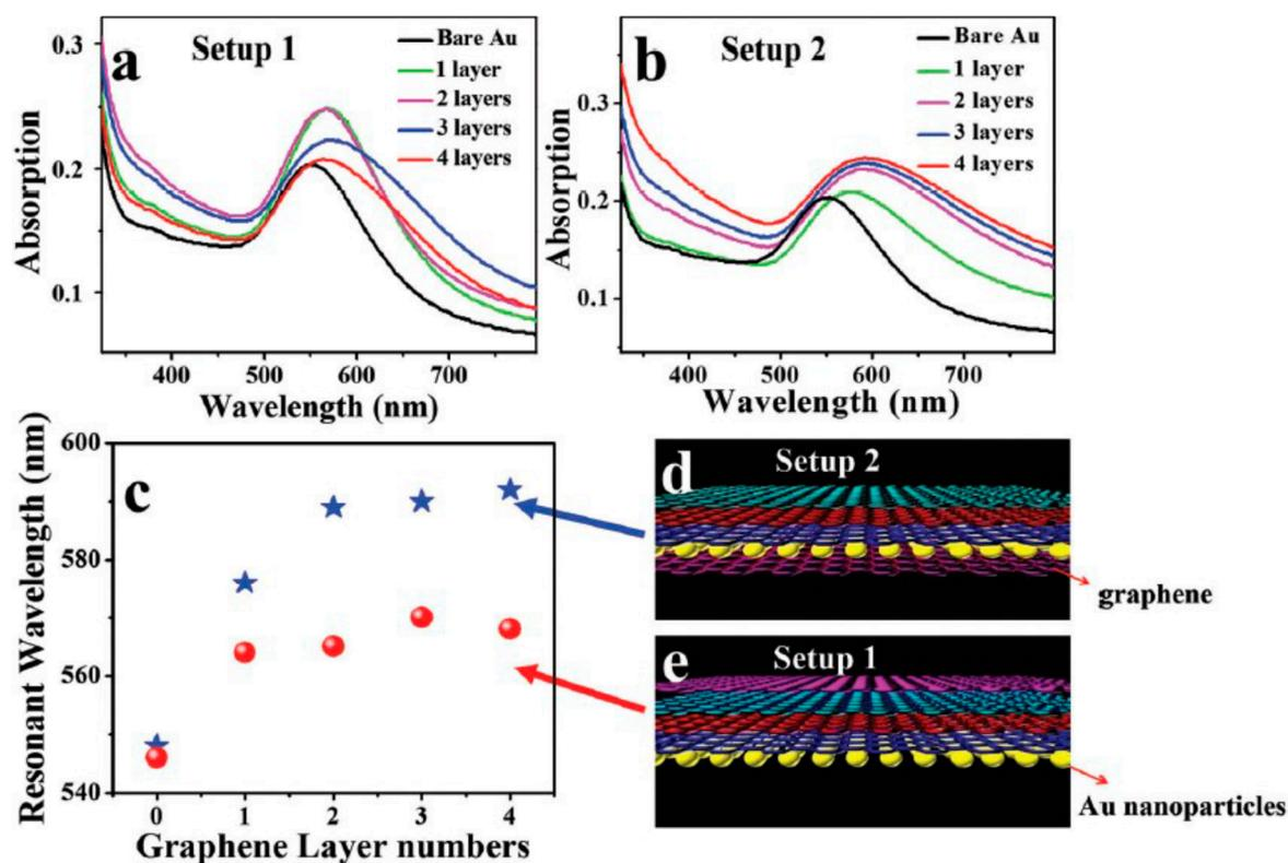
**Figure 3.** Absorption spectra of gold NPs coated (a) and encapsulated (b) by graphene layers. (c) Gold NP LSPR wavelengths for Setups 1 and 2. (d,e) The structures of the setups used in (b,a) [67].
