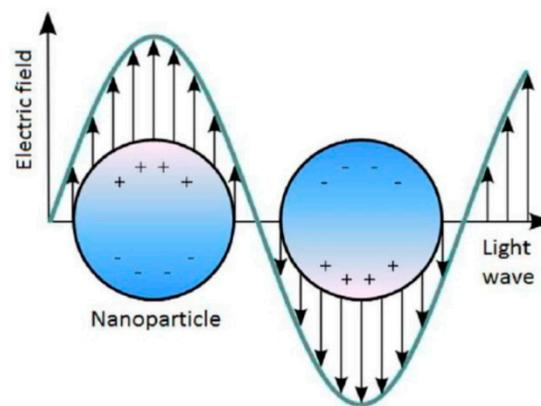
Figure 1. Metal NP external electric field interaction [17].
