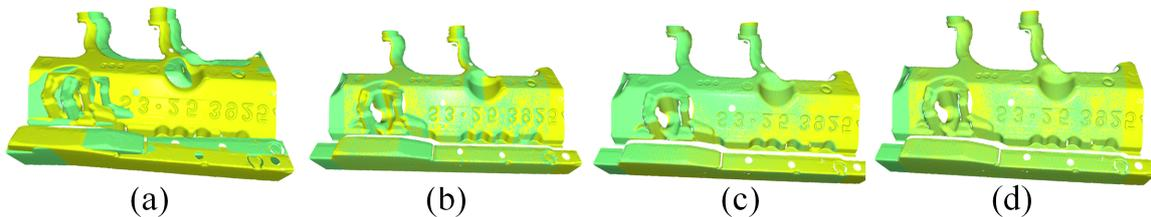
**Figure 3.** (a) Initial relative pose between source (green) and target (yellow) point cloud, (b) Registration result by only minimizing geometric error in Equation (8), (c) Point-to-plane ICP performed on 3D point cloud with a max distance threshold to eliminate outliers, (d) Minimizing both of the geometric error and curvature error as proposed in this paper.
