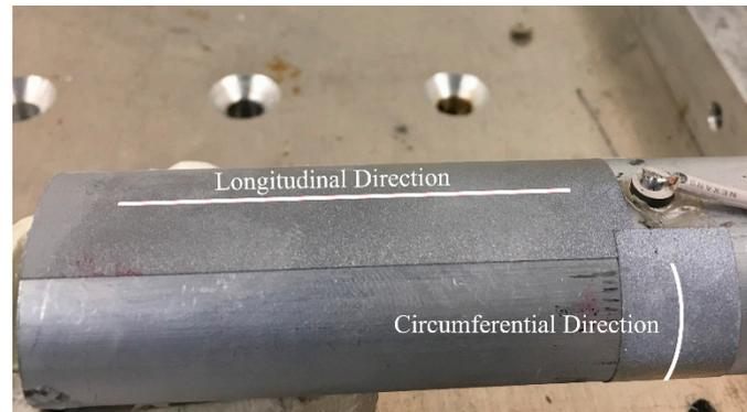
**Figure 6.** Image of oval surrogate bone with showing the longitudinal and circumferential scan line.
