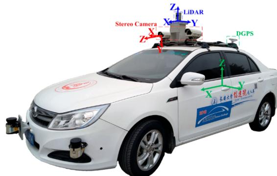
**Figure 9.** Autonomous vehicle platform. Reproduced from Zhao, X.; Min, H.; Xu, Z.; Wang, W. *An ISVD and SFFSD-based vehicle ego-positioning method and its application on indoor parking guidance. Transportation Research Part C: Emerging Technologies*, 2019; 108: 29–48. Copyright © 2019 Elsevier Masson SAS. All rights reserved [33].
