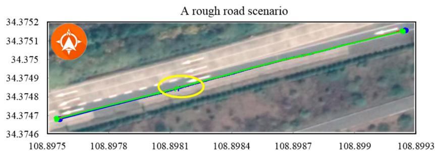
**Figure 20.** Scenario involving violent shaking on a rough road. The shaking movement affected the IMU-based or in-vehicle sensor-based positioning, and the maximum error was approximately 1.2 m, as indicated by the yellow circle.
