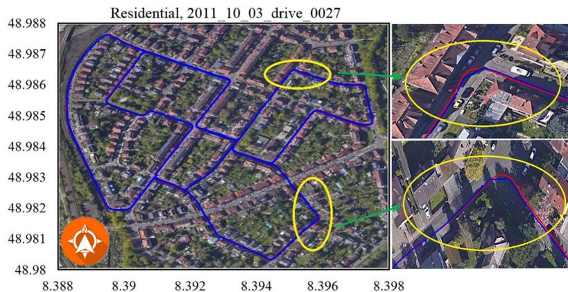
**Figure 12.** Residential, 2011\_10\_03\_drive\_0027. There was an error in the trajectory because the car moved into a cluttered environment, and the GPS signal was blocked or had a multipath effect.
