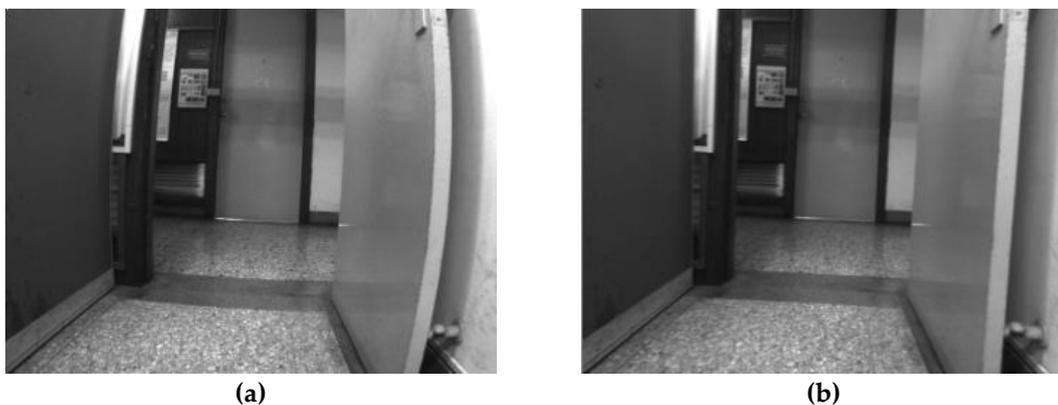
**Figure 2.** (a) Distorted image and (b) its correction.
