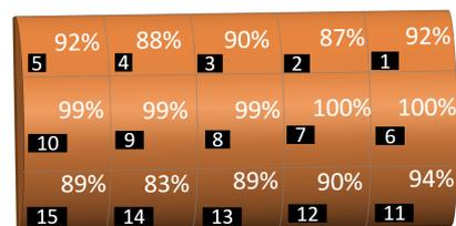
**Figure 9.** Contact localisation accuracy for individual grid cells of the sensor with contact forces in normal and non-normal directions using 2 mm and 6 mm probes.
