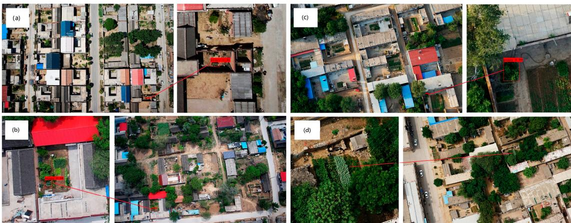
**Figure 15.** Partial test results for complete unmanned aerial vehicle (UAV) images: (a,b) the true detection; (c) false detection; (d) missed detection.
