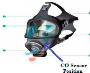
Figure 4. The position of CO sensor on the mask.
