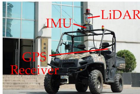
Figure 17. The vehicle used in experiments on rough terrain.
