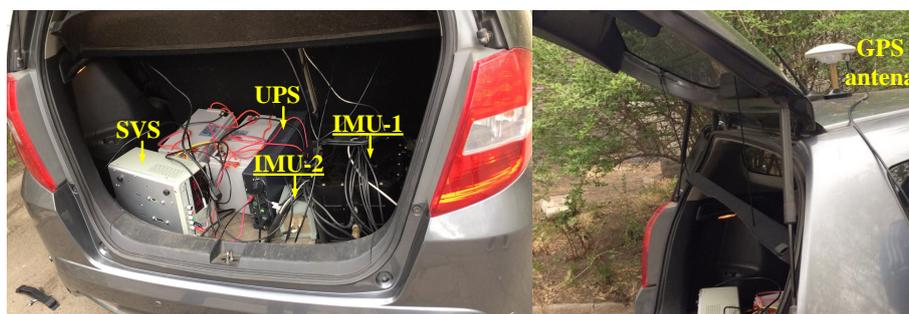
**Figure 11.** The vehicle experimental device.
