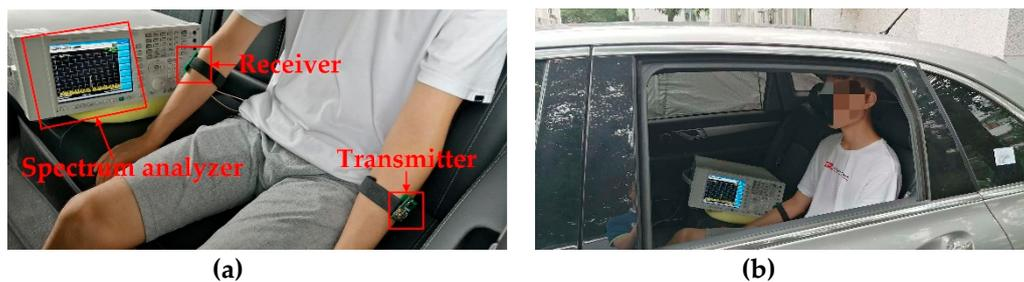
**Figure 11.** An illustration of the experimental setup in the in-vehicle scenario. (a) the local scenario; (b) the whole scenario.
