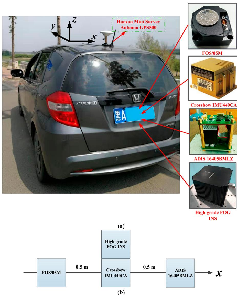
**Figure 4.** The equipment installation diagram for the road test. (a) The test vehicle and sensors; (b) internal installation diagram.
