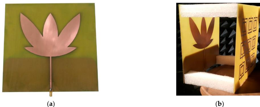
**Figure 27.** Manufactured bio-inspired PMA: (a) without metamaterial superstrate [26]; (b) with metamaterial superstrate.
