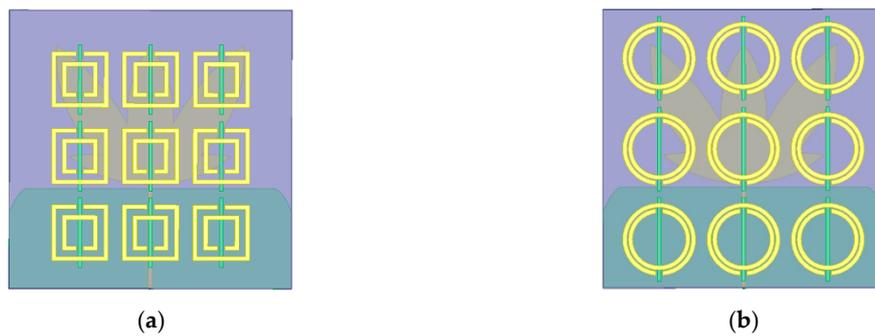
**Figure 9.** Metamaterial superstrates positioned over the bio-inspired PMA: (a) rectangular; (b) circular.
