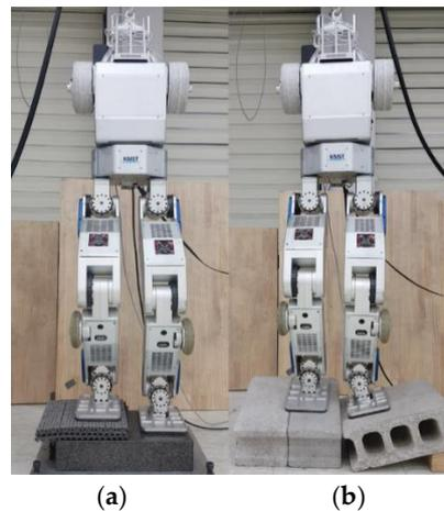
**Figure 12.** Leg length and foot orientation control on uneven terrain. (a) Height difference and (b) both height and orientation difference.
