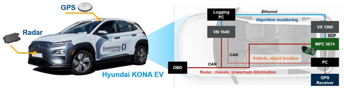
Figure 2. Vehicle configuration.
