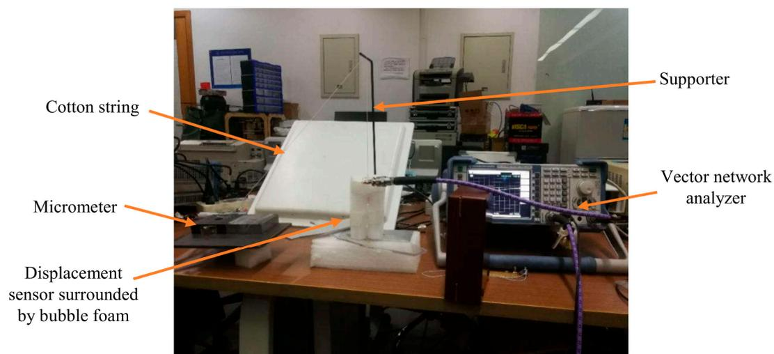
**Figure 12.** The experimental setup.
