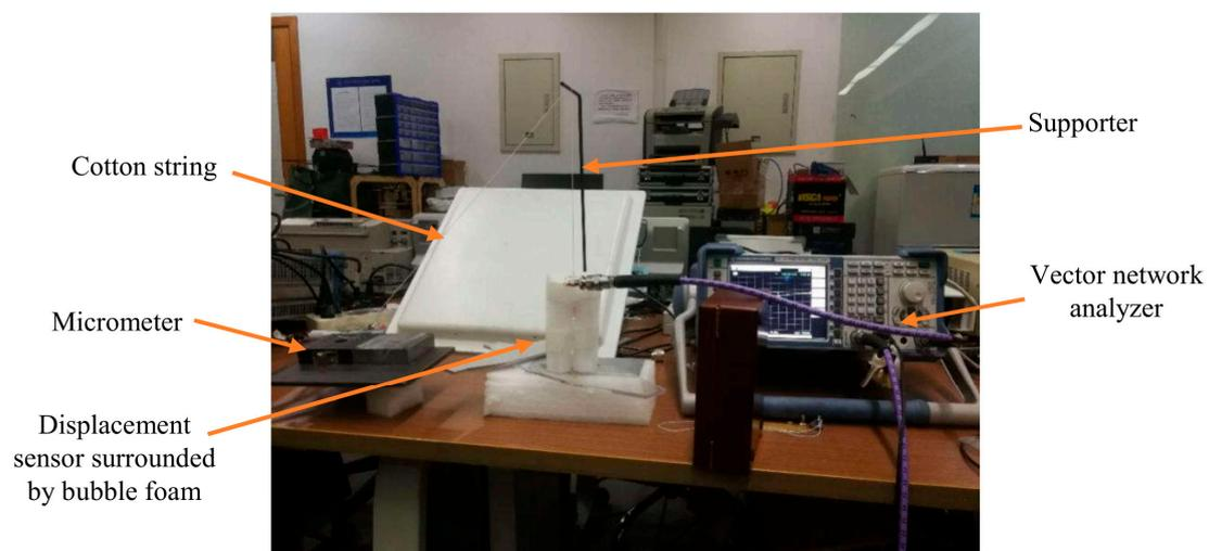
**Figure 12.** The experimental setup.
