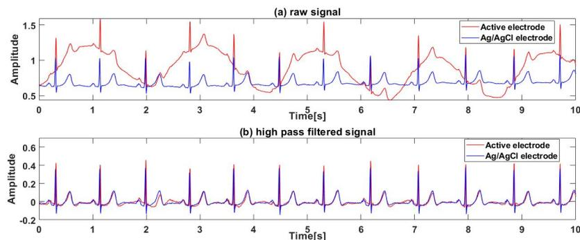
**Figure 6.** Comparison between signals measured by active electrodes and Ag/AgCl electrodes: (a) raw signal, (b) high pass filtered signal.
