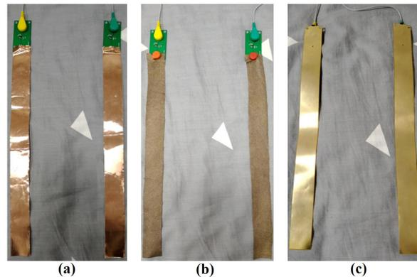
**Figure 2.** Three pairs of electrodes made of different materials: (a) copper foil tape, (b) conductive textile, (c) FPC.
