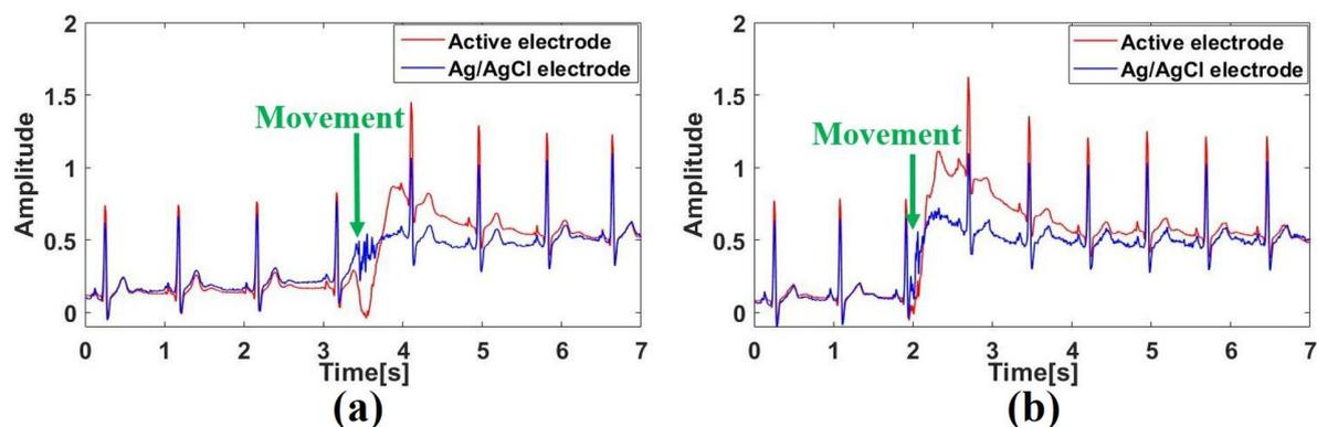
**Figure 8.** ECG measurement under turning movement of upper body: (a) left turning movement of upper body, (b) right turning movement of upper body.
