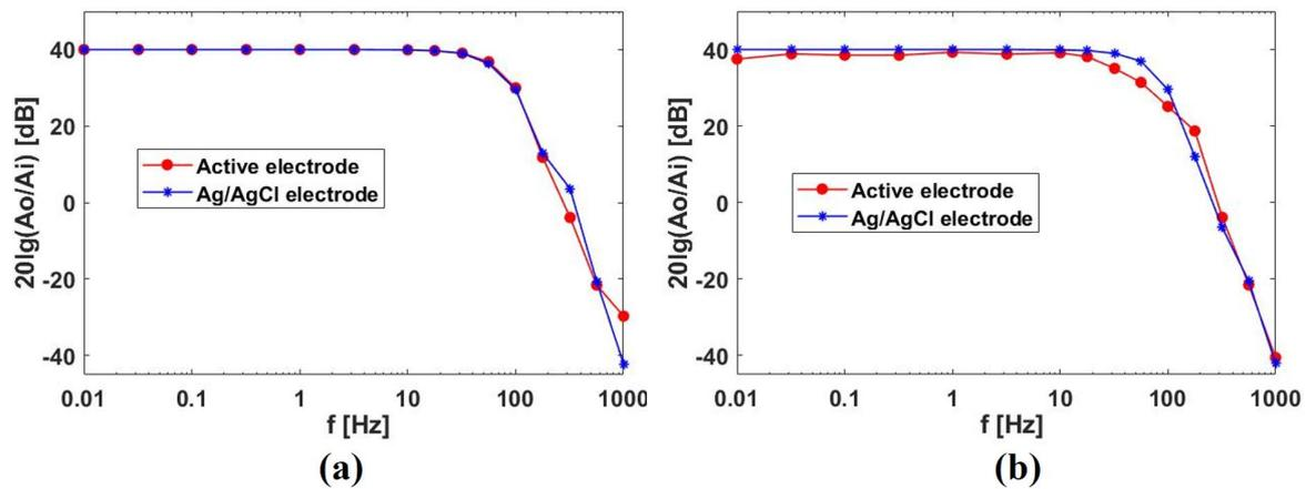
**Figure 9.** Amplitude-frequency response of active electrode system and passive electrode system: (a) electrodes of the active electrode system measure signals directly, (b) electrodes of the active electrode system measure signals through clothes (a simple cotton underwear about 1 mm in thickness).
