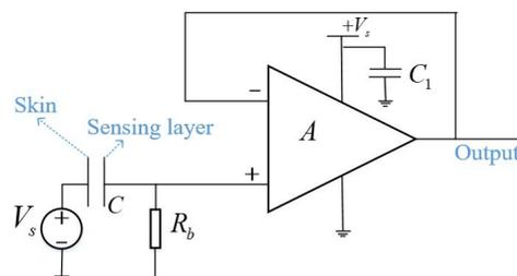
**Figure 1.** Equivalent electronic circuit of the active electrode.
