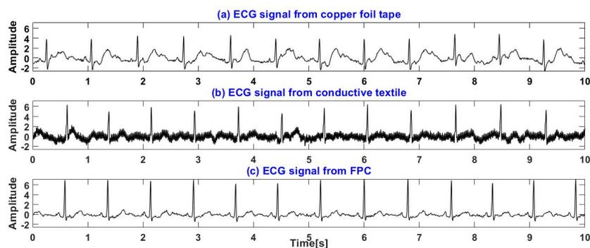
**Figure 14.** ECG signals of a subject sitting on a chair: (a) ECG signals measured by copper foil tape. (b) ECG signals measured by conductive textile. (c) ECG signals measured by FPC.
