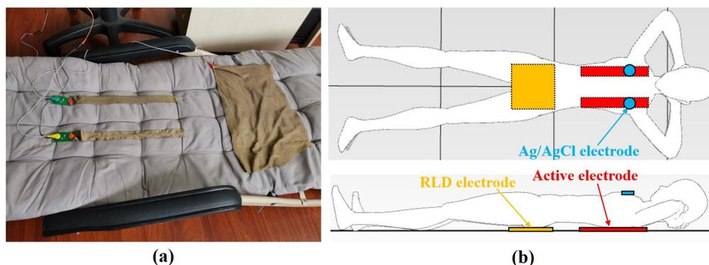
Figure 12. Experimental setups in lying supine posture: (a) picture, (b) schematic.
