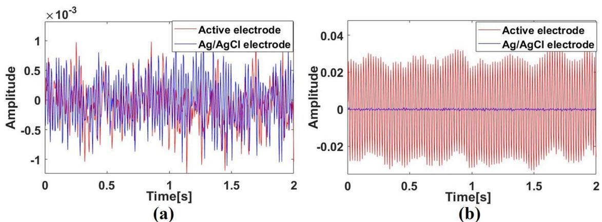
**Figure 10.** Output noise of system under short connection of electrodes: (a) electrodes of the active electrode system short connect directly, (b) electrodes of the active electrode system short connect through clothes (a simple cotton underwear about 1 mm in thickness).
