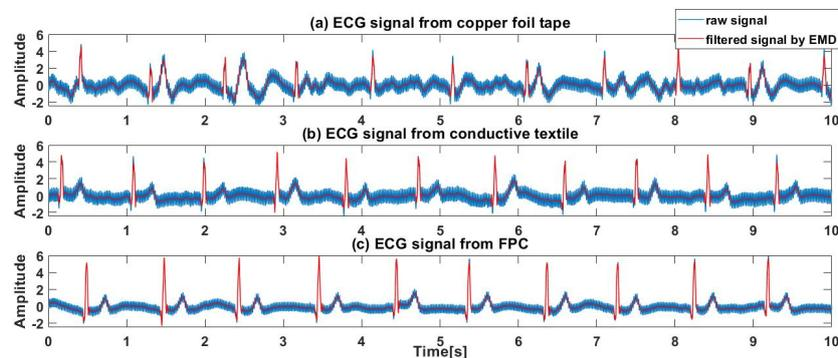
**Figure 16.** ECG signals of a subject side lying on a recliner: (a) ECG signals measured by copper foil tape. (b) ECG signals measured by conductive textile. (c) ECG signals measured by FPC.
