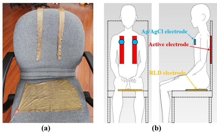
Figure 11. Experimental setups in sitting posture: (a) picture, (b) schematic.
