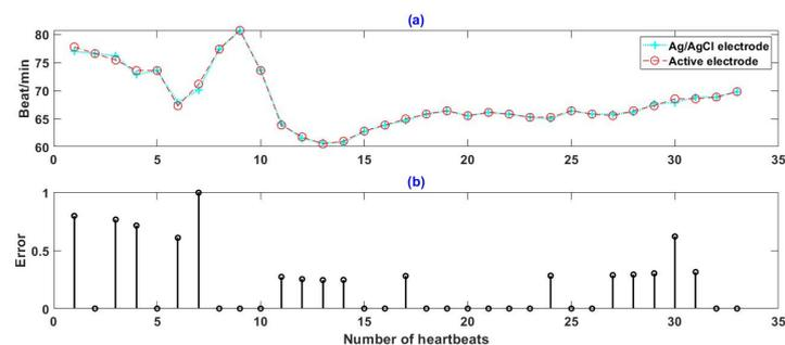
**Figure 7.** Comparison between instantaneous heart rate obtained by active electrode and Ag/AgCl electrode: (a) instantaneous heart rate, (b) the error between instantaneous heart rate obtained by two kinds of electrode.
