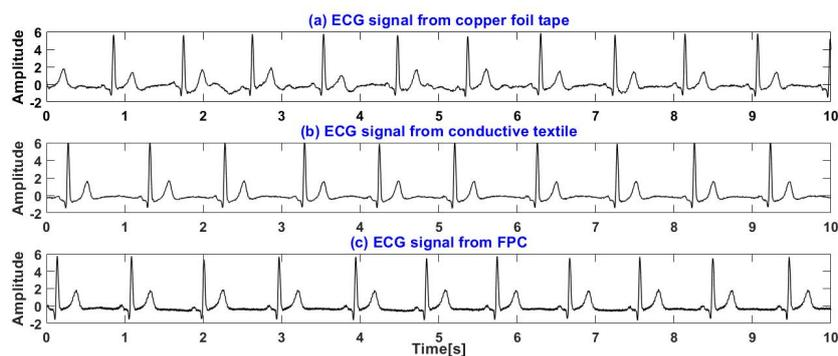
**Figure 15.** ECG signals of a subject lying supine on a recliner: (a) ECG signals measured by copper foil tape. (b) ECG signals measured by conductive textile. (c) ECG signals measured by FPC.
