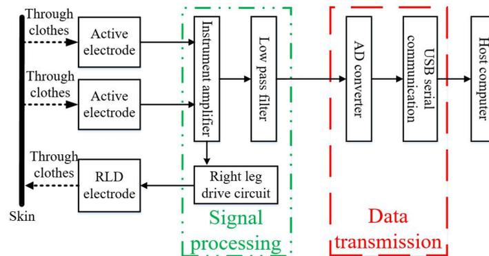
Figure 3. Hardware system block diagram.
