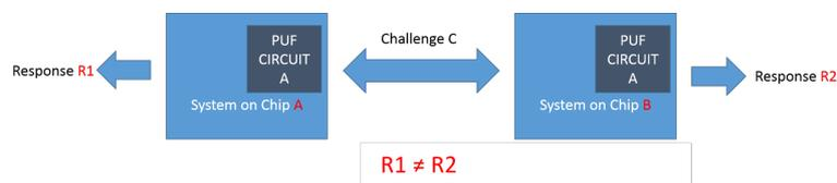
**Figure 1.** Two identical physical unclonable functions (PUFs) circuits on two different chips generate different responses.
