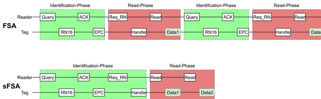
Figure 5. Comparison of the streaming procedure using the standard EPC C1G2 on top of the figure, and the proposed approach below for  $N = 1$  and  $S = 2$ .
