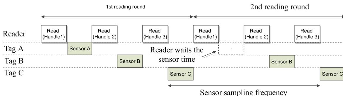
**Figure 4.** Example of two Read rounds using sensor Frame Slotted Aloha protocol (sFSA) ( $N = 2$ ,  $S = 2$ ).
