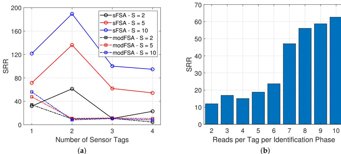
Figure 11. Results of the comparison between the modified FSA (modFSA) and the sFSA protocol with varying tags and reads per tag. (a) Comparison of SRR between the modFSA and sFSA with  $N = 1, 2, 3, 4$  tags and  $S = 2, 5, 10$  reads per tag. (b) Variation of the number of reads per tag in the Sense phase with  $N = 3$ .
