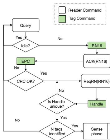
Figure 6. Identification Phase of sFSA using the unique handle procedure.
