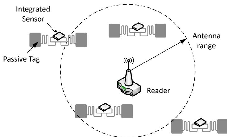
**Figure 1.** Example of a Radio Frequency Identification (RFID) sensor network [8].
