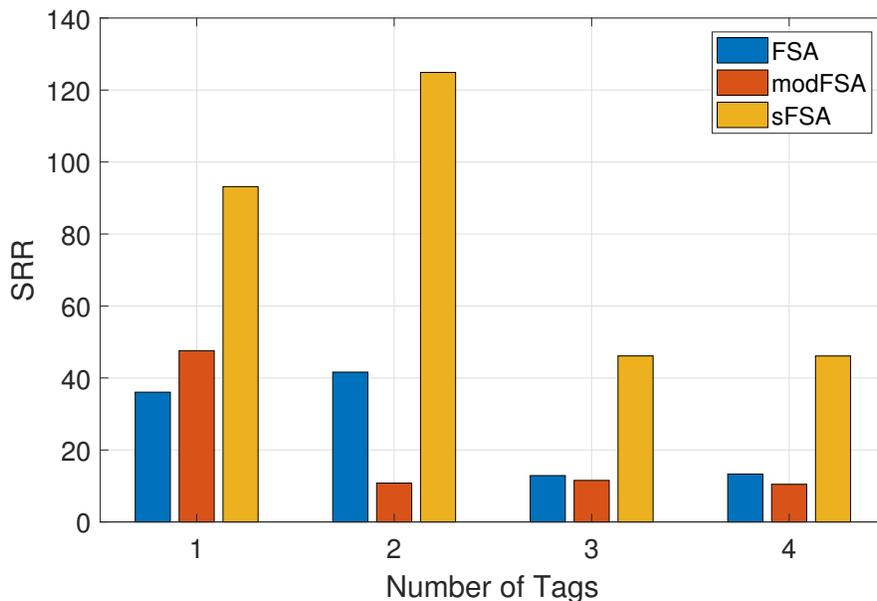
Figure 10. Comparison of SRR for the Framed Slotted Aloha (FSA), the modified FSA and the sFSA protocols for  $N = 1, 2, 3$  tags and  $S = 5$  reads per tag.
