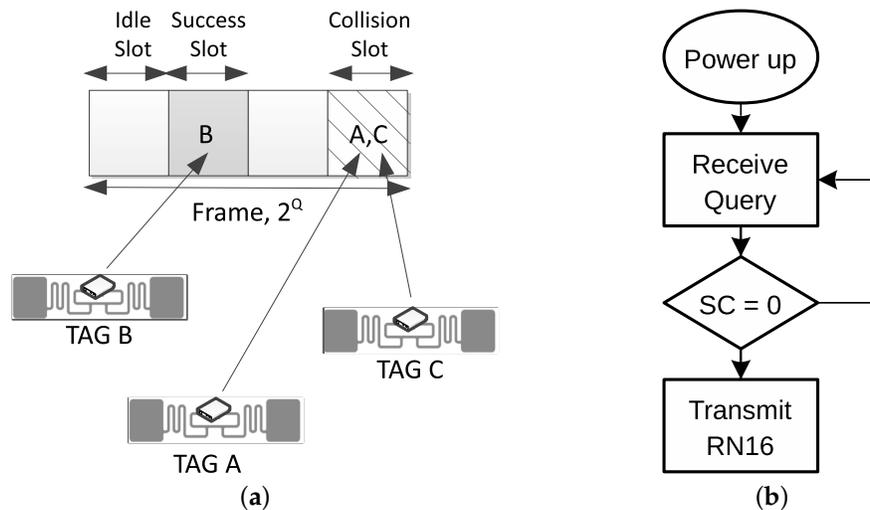
**Figure 2.** EPC C1G2 definition and slot selection process [8]. (a) Slot definitions for EPC C1G2 Identification Phase; (b) Tag response procedure to Query command.
