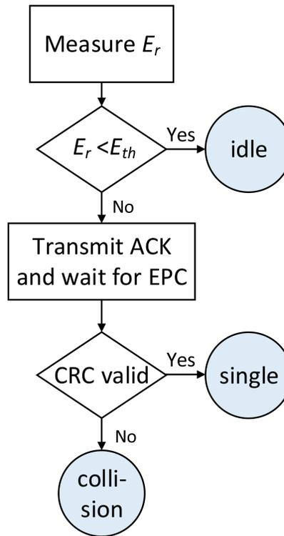
**Figure 8.** Flow diagram to differentiate the types of tag responses.
