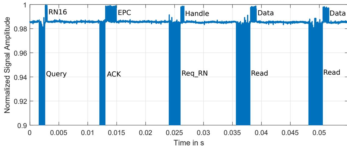
**Figure 9.** Three consecutive *Read* commands and three Wireless Identification and Sensing Platform (WISP) accelerometer tag responses.
