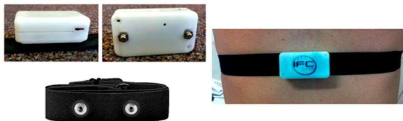
**Figure 1.** Wearable sensor for electrocardiographic (ECG) signal acquisition based on ECG SHIMMER<sup>TM</sup> device.
