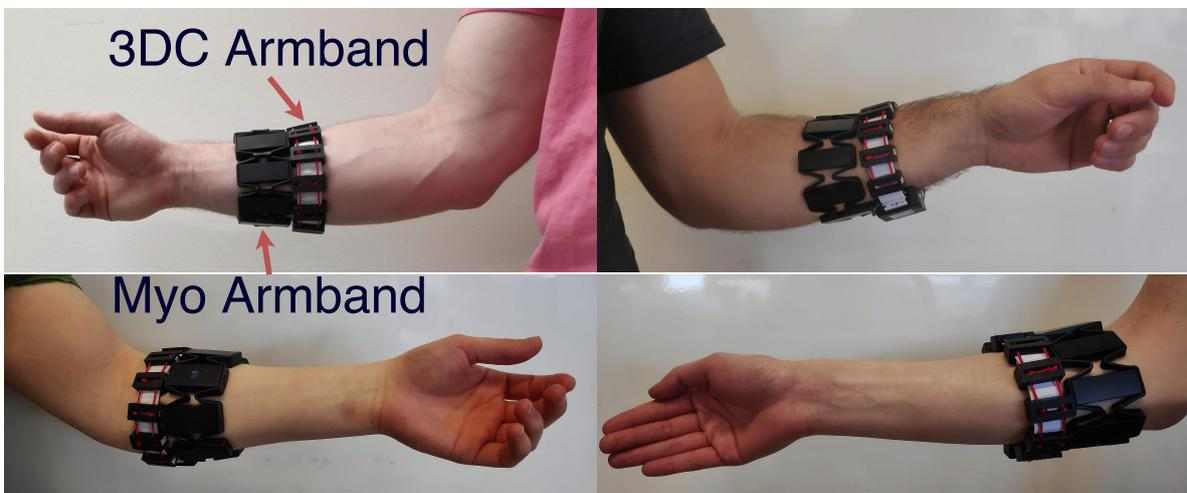
**Figure 6.** The two different armband configurations (left/right) employed in this work with the 3DC being either above or below the Myo armband with respect to the participant’s wrist. This figure also showcases the wide variety of armband positions recorded in the proposed dataset.
