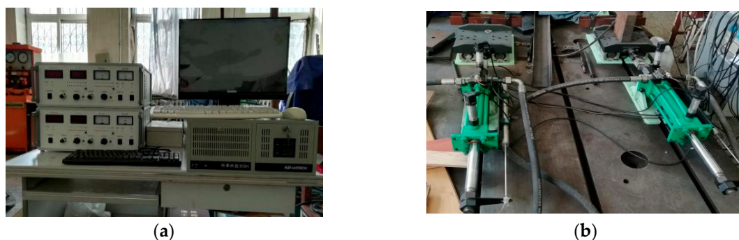
Figure 9. The electro-hydraulic semi-physical experiment platform. (a) Experiment platform. (b) Electro-hydraulic servo system.
