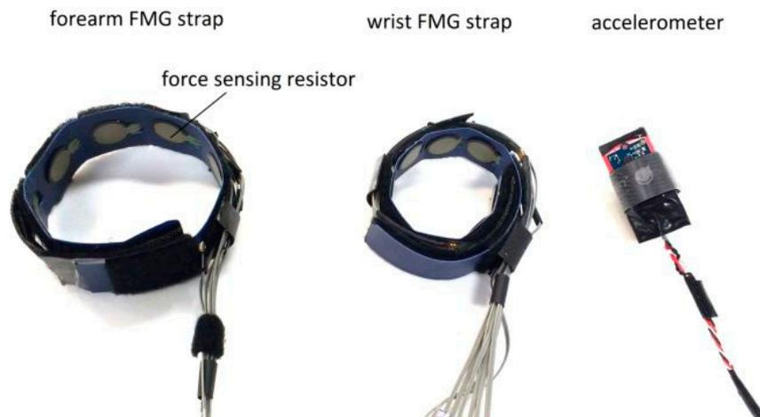
**Figure 2.** FMG and motion sensing devices.
