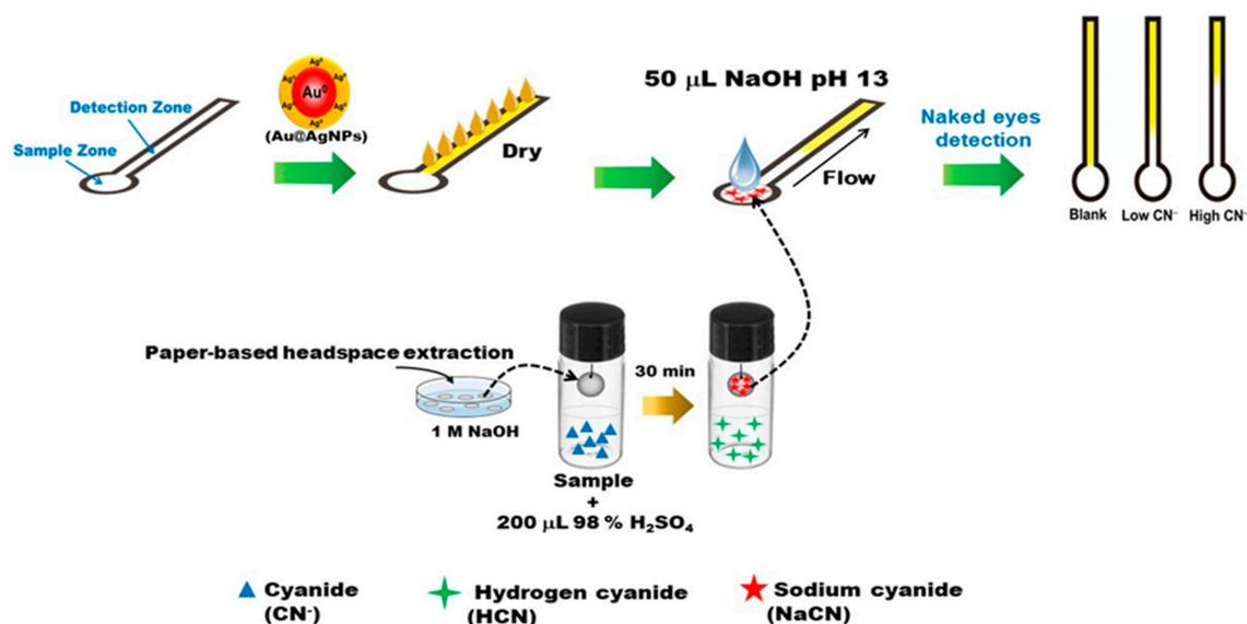
**Scheme 1.** Schematic design of the distance-based paper sensor designs and general analytical methods.
